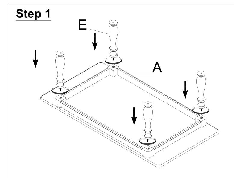
NOTE, WAIT TO TIGHTEN ALL COMPONENTS COMPLETELY UNTIL UNIT IS FULLY ASSEMBLED. THIS WILL ALLOW FOR EASIER ASSEMBLY.
