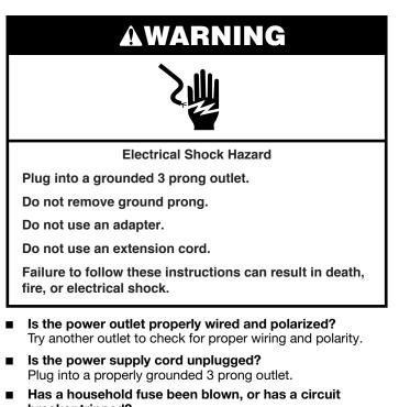
**breaker tripped?** Replace the fuse or reset the circuit breaker. If the problem continues, call an electrician.
