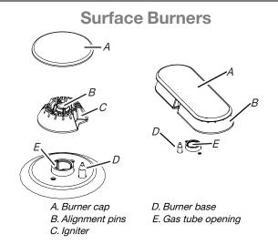
**IMPORTANT:** Do not obstruct the flow of combustion and ventilation air around the burner grate edges.
