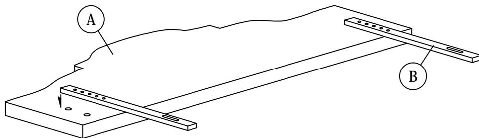
Align pre-drilled support stand holes over the pre-drilled headboard holes according to your desired headboard height
