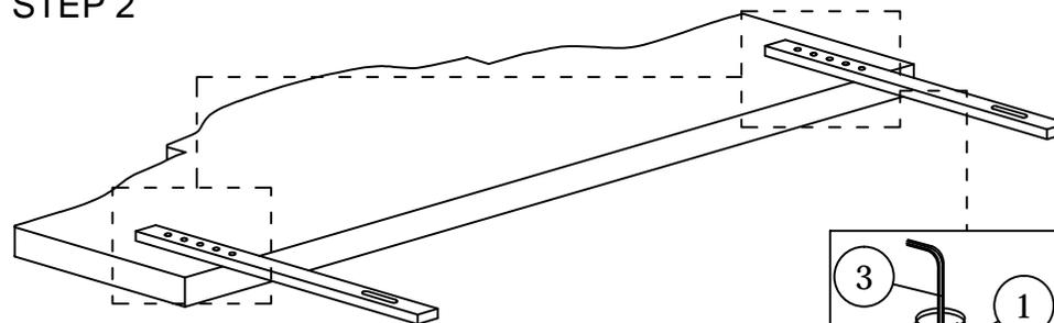
Secure each support stand by using 2x JCBB Bolt [1] and 2x M8 Flat Washer [2].
