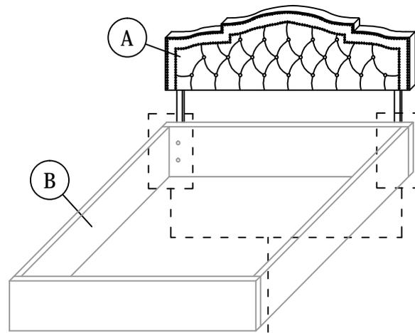
1. Line up the bed frame board's pre-drilled holes to match those of the headboard.
