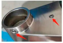
5. Lay the door handle against to the oven door and fit it on the connection part, and use the wrench to get the door handle holder tight;
