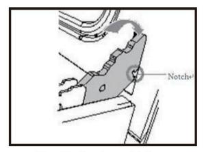
2. Insert the hinge tongues into the slots making sure that the notches on both sides drop into place as shown.
