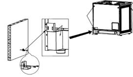
Attach bracket with mounting hardware provided.
