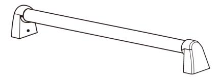
4. Secure the oven handle with two screws on each door handle holder (if not, handle might be loose)
