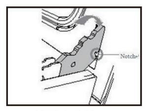
Hold the door firmly in an approximately open position.
