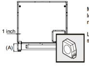
Measure from floor to bottom of the anit-tip opening located on the back of range. This will be measurement (A).
