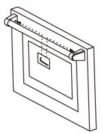
6. Use the wrench to tighten the door handle holders.
