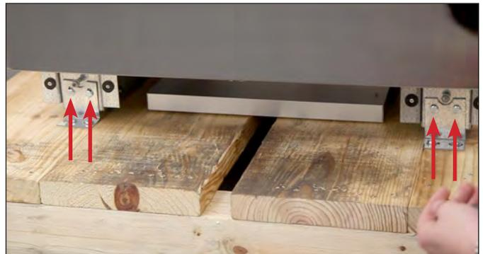
**FIG. 7.** Shipping bracket bolt locations.
