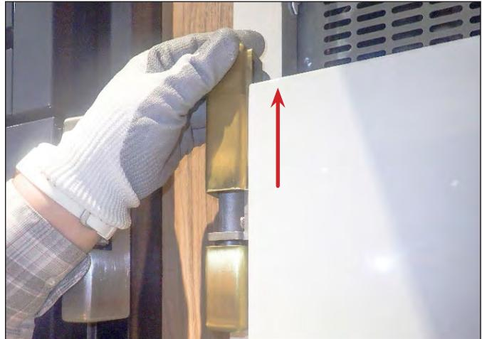
FIG. 2. Remove the hinge covers.
