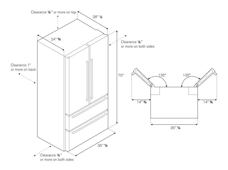
INSTALLATION: There shall be a space not less than 1/8 inch from the top of your refrigerator, not less than 1/8 inch from both sides and not less than 1 inch from the back of the refrigerartor to the adjacent walls respectively. This requirement is necessary to create clearance in order to open and close the door as well as to avoid the spacing for adequate ventilation around the refrigerator.
