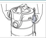
**2.** Undo clips on both sides of top cover.
