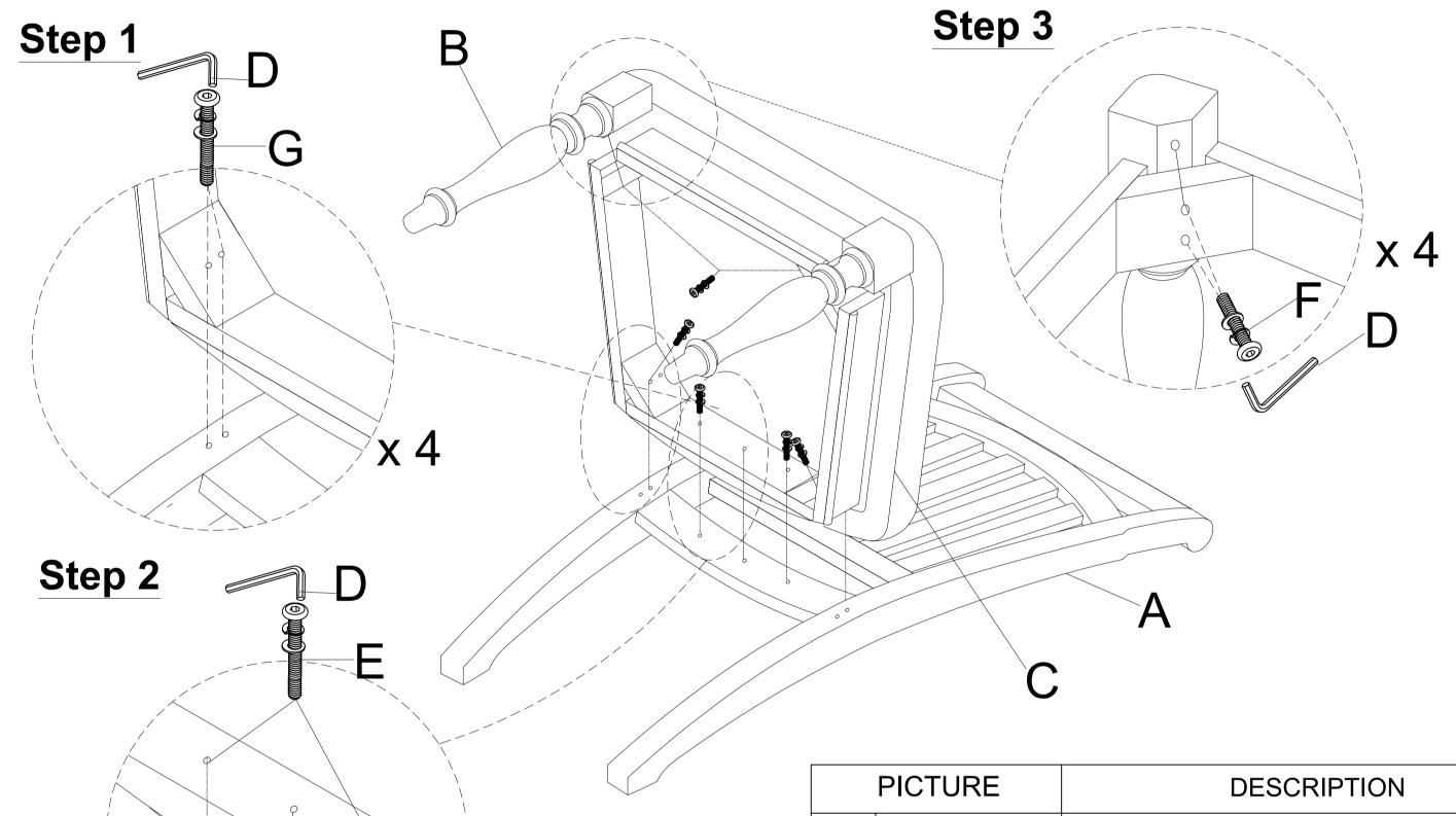
PLEASE DO NOT TIGHTEN THE BOLTS UNTIL ALL THE PARTS ARE IN POSTION
