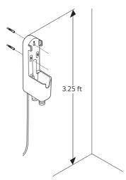
Attach the charging station to the wall with the wall anchoring screws.
