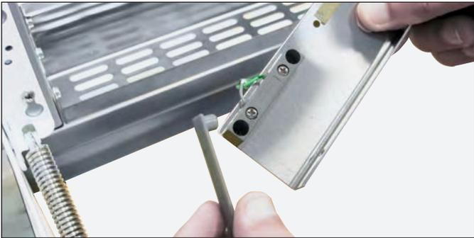
FIG. 4. Remove the plastic cover.
