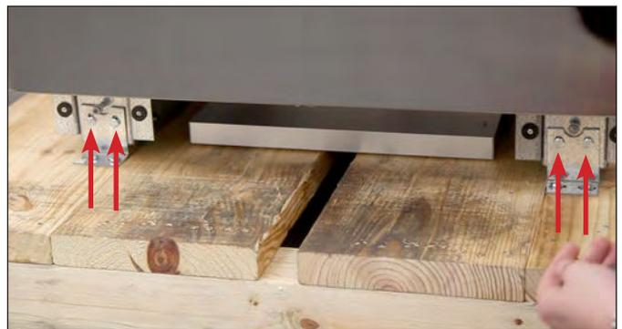
**FIG. 7.** Shipping bracket bolt locations.
