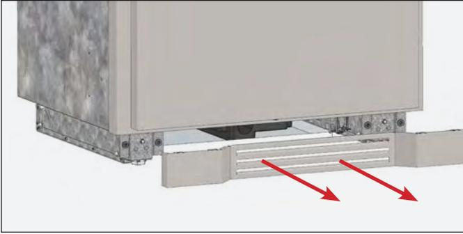
FIG. 1. Pull the kickplate from the cabinet.
