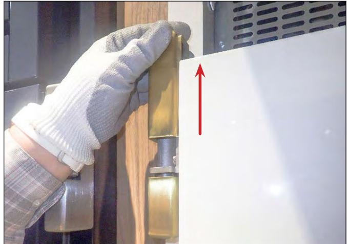
FIG. 2. Remove the hinge covers.
