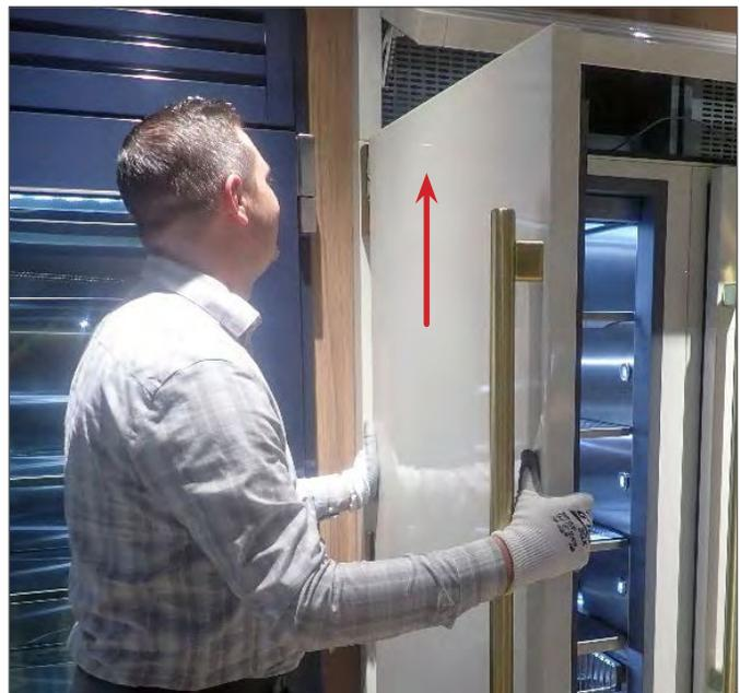
FIG. 3. Remove the door.
