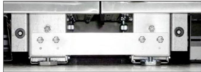
**FIG. 18.** Installed joining bracket.
