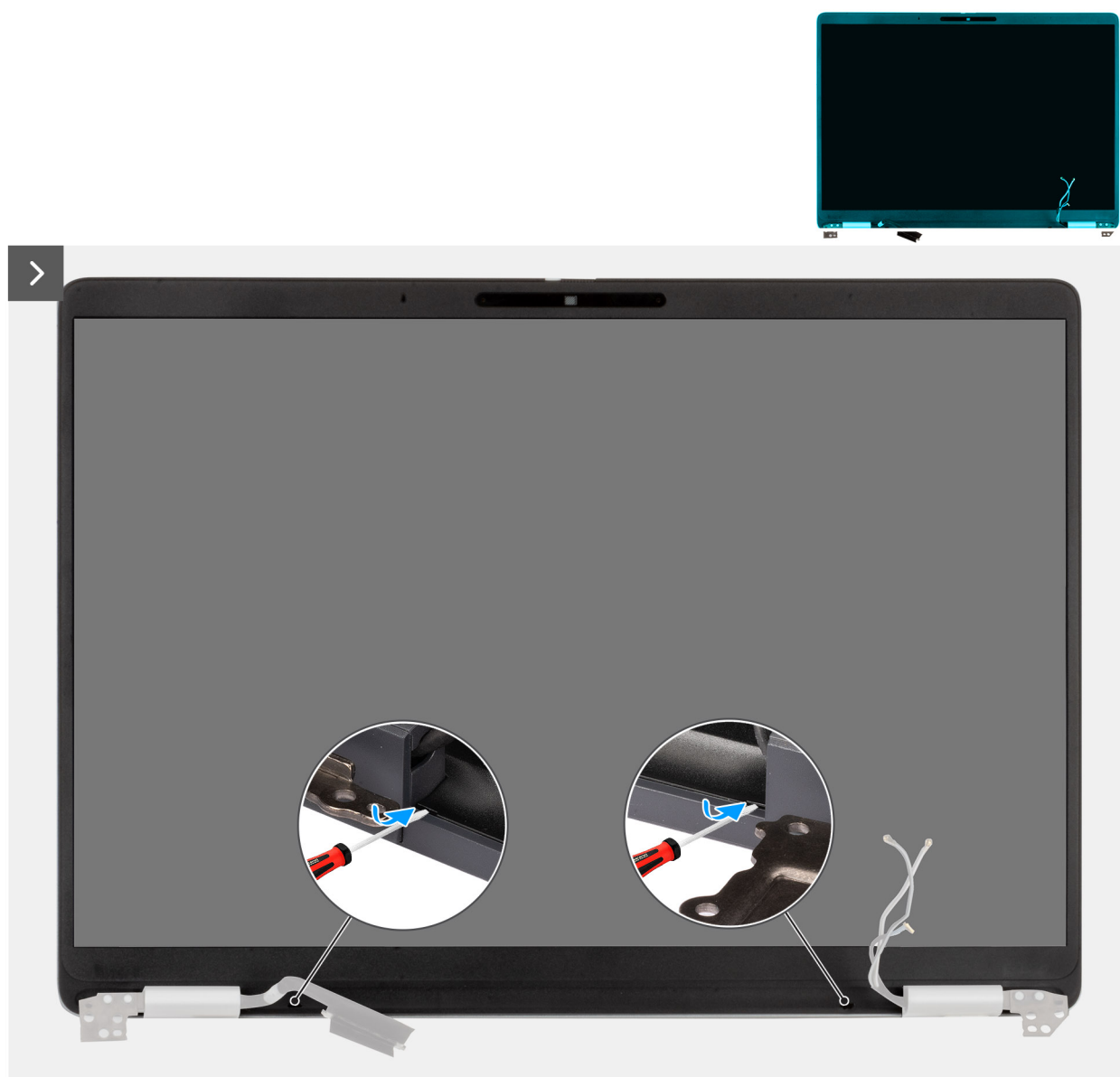
Figure 68. Removing the display bezel
