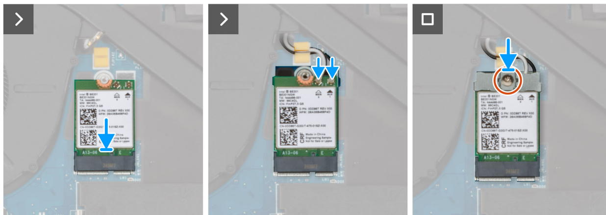
Figure 41. Installing the WLAN card
