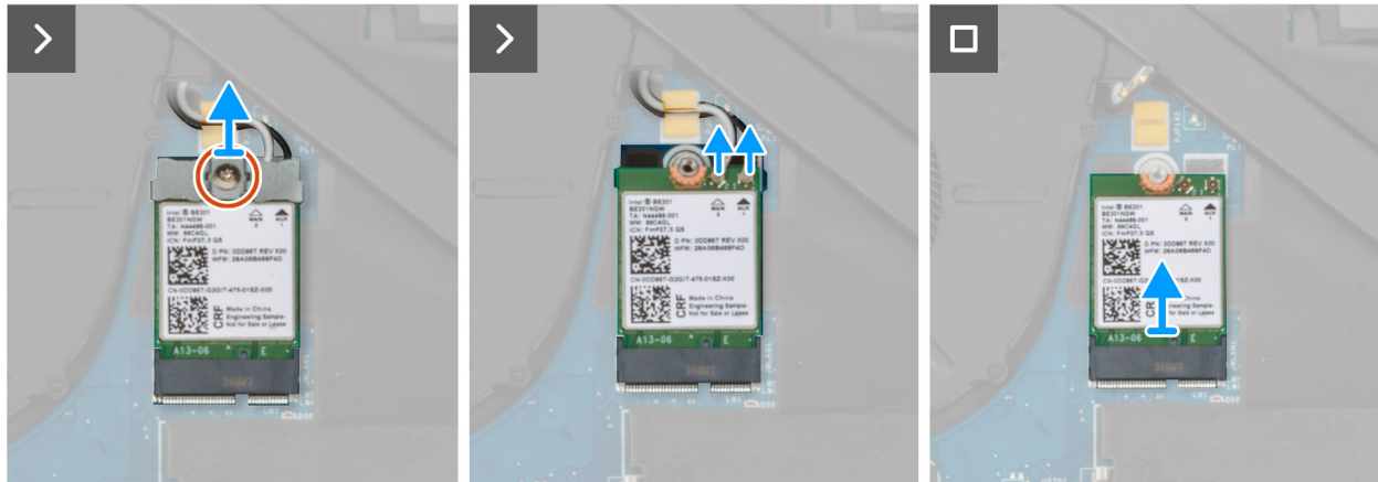
Figure 40. Removing the WLAN card
