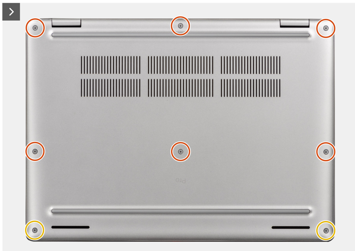
Figure 22. Removing the base cover
