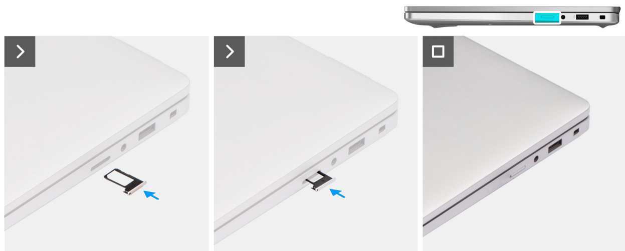
Figure 21. Installing the SIM-card tray
