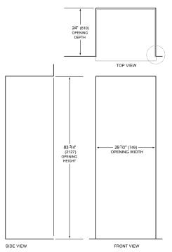
NOTE: 3<sup>1</sup>/2" (89) finished returns will be visible and should be finished to match cabinetry Shaded line represents profile of unit.
